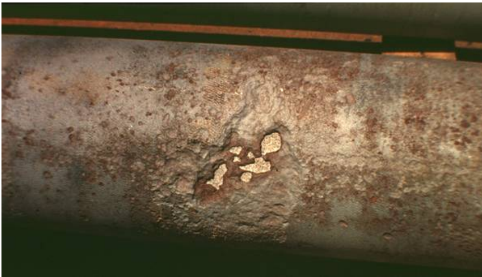
Figure 20 Vancouver, BC, Polyethylene-encased Ductile Iron Pipe After Sandblasting Where Graphitization and Cement Mortar Lining Previously Held 650- PSI Water Pressure
