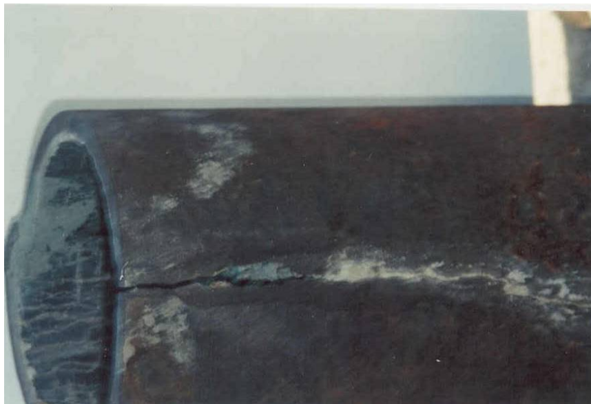
Figure 6 Sheridan Deep Graphitization Corrosion Along Crack on Ductile Iron Pipe in Less Than 15 Years
