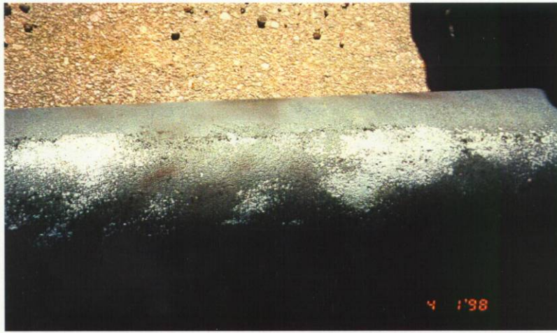
Figure 28 Colorado Springs, Colorado, Sewer Force Main With Uniform Pitting on Pipe Bottom from MIC Corrosion
