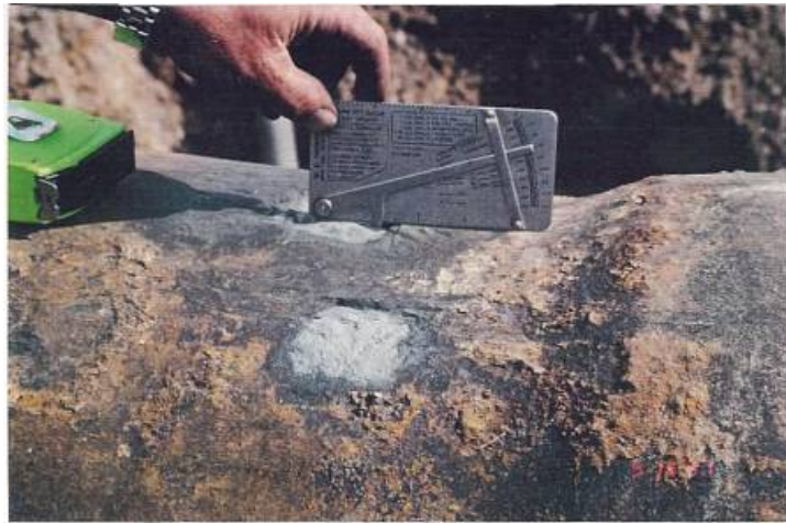
Figure 4 Sandblasted 24-Inch 33-Year-Old Ductile Iron Corrosion With 3/16-Inch Surface Graphitization Layer
