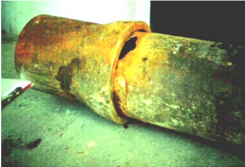
Figure 34 California City, California Corrosion Leak on Cathodic Protected Polyethylene Encased 14-inch Ductile Iron Pipeline
