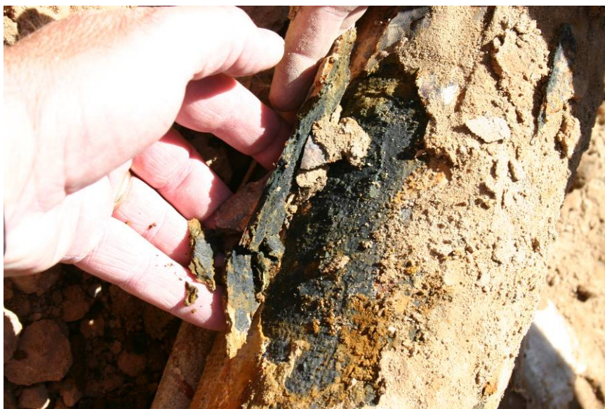
Figure 32 Vernal, Utah, CP Polyethylene-Encased DIP with Black Layer and Graphitization Under Polyethylene Encasement
