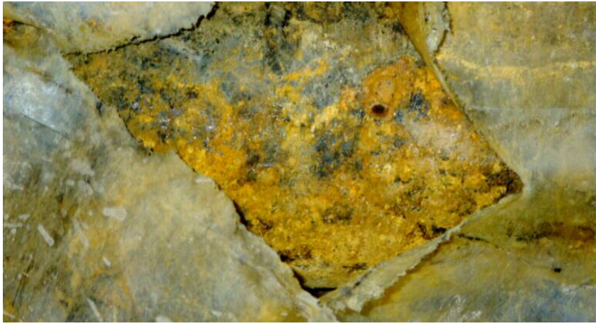
Figure 33 Sheridan, Wyoming, Surface Corrosion Indicating Possible Electrical Shielding Of Cathodic Protection With Loose-Bonded Polyethylene Encasement
