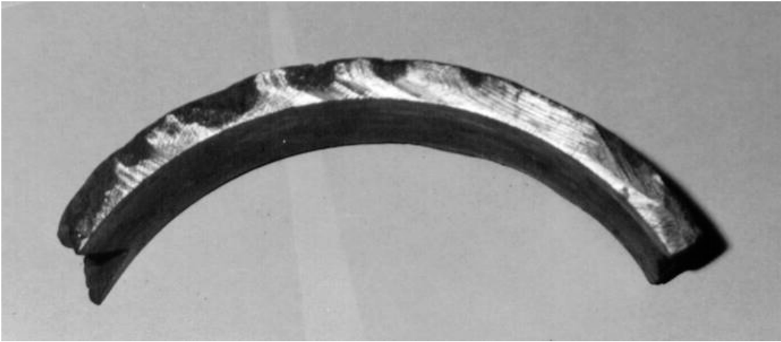
Figure 2 Soft Black Graphitization Pockets Visible on Pipe Edge When Cut
