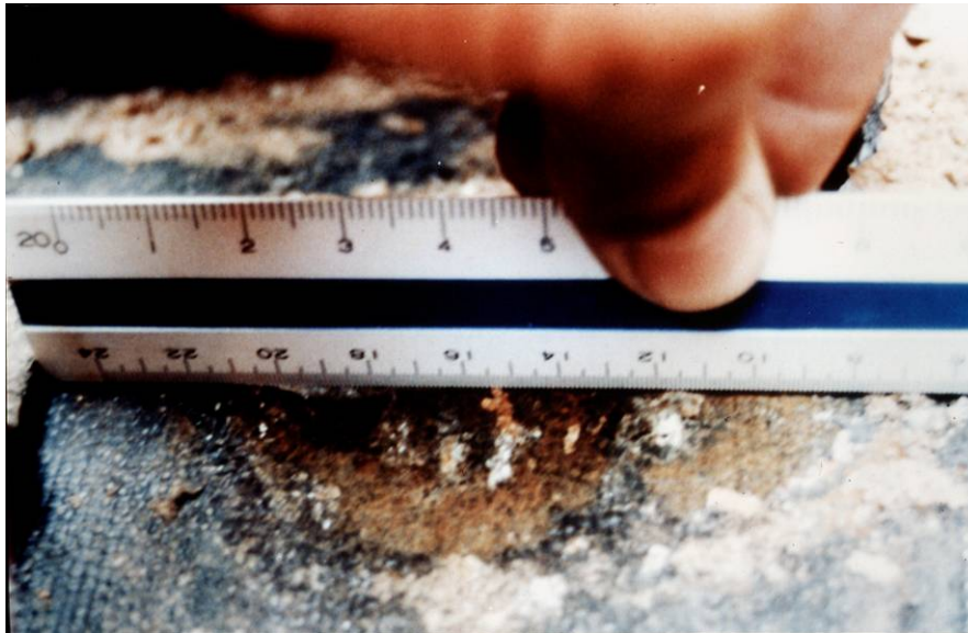
Figure 31 Vernal, Utah, 125-Mil, (0.3175 cm)-Deep Corrosion on CP Polyethylene-Encased DIP
