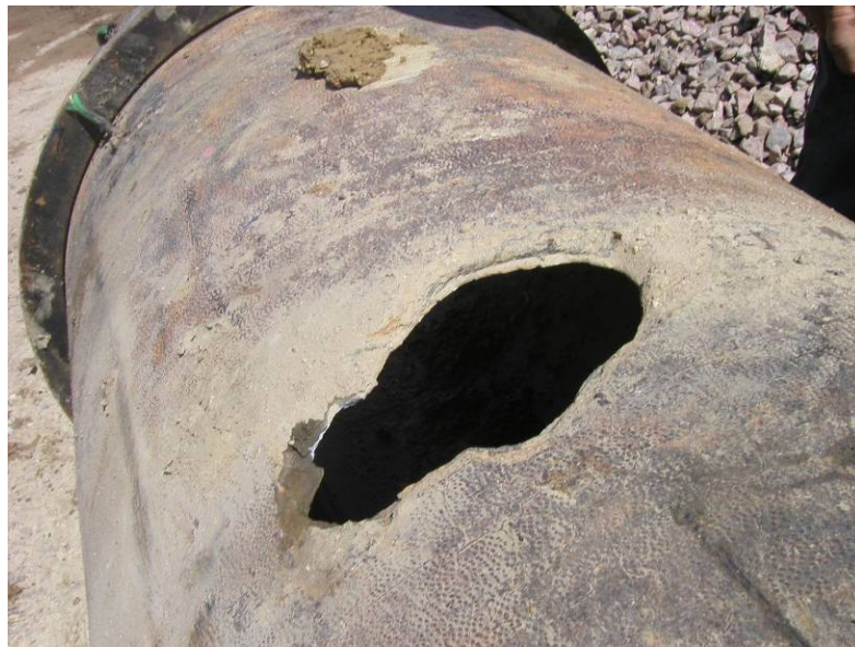
Figure 11 Colorado Corrosion Damage Repair Required Removal of Five-Foot Section of Polyethylene-encased Ductile Iron and Replacement with New Pipe with Galvanic Anodes
