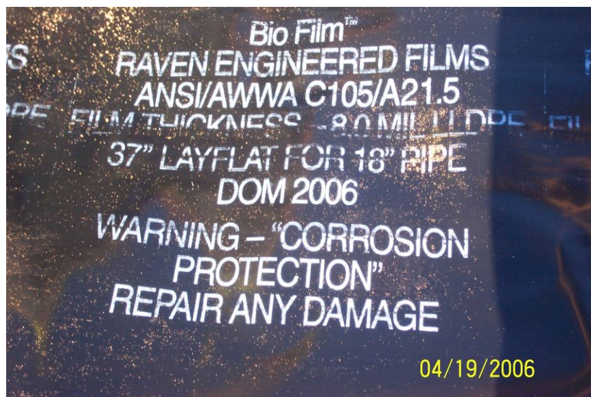
Figure 43 2006 Minnesota Forcemain Project Anti-MIC 8-mil Linear Low Density Polyethylene Encasement With Warning
