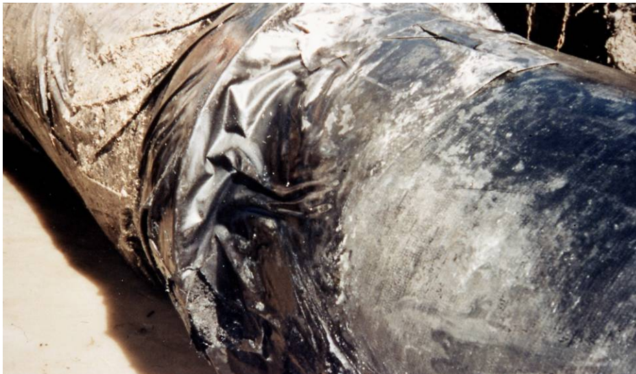
Figure 21 Sheridan, Wyoming, Ductile Iron Polyethylene Encasement Folded and Taped In Place, With No Encasement Damage Visible
