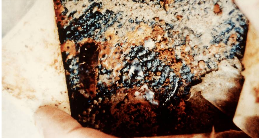
Figure 30 Vernal, Utah, Electrical Shielding Of 10-Year Old Cathodic Protected Pipeline With 30- to 60-mil Deep Pipe Under Intact Polyethylene Encasement
