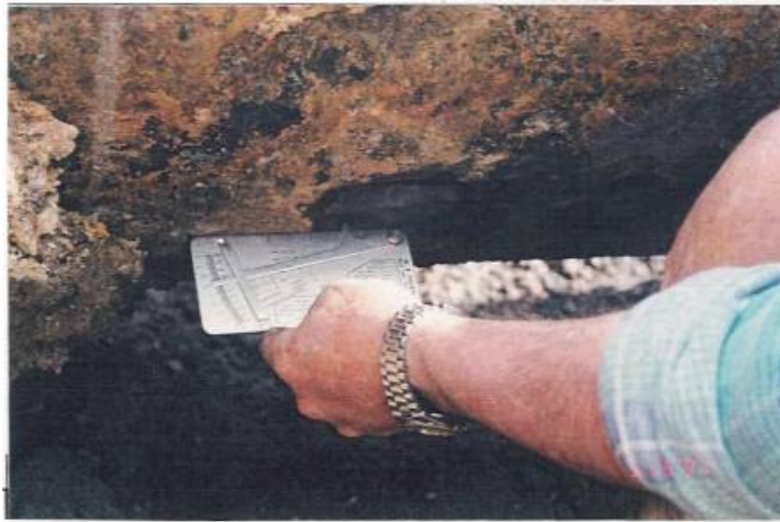
Figure 5 24-inch 33-Year-Old Ductile Iron Pipe with 2-inch by 3-inch Sized 0.310-mils Deep (75 Percent of Pipe Wall) Plug-Type Corrosion With Some Surface Graphitization
