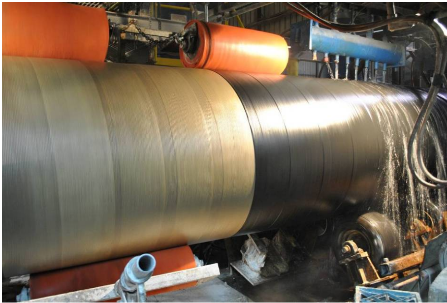
Figure 51 External Polyethylene Ductile Iron Coating Internal and External Coating with Water Quench
