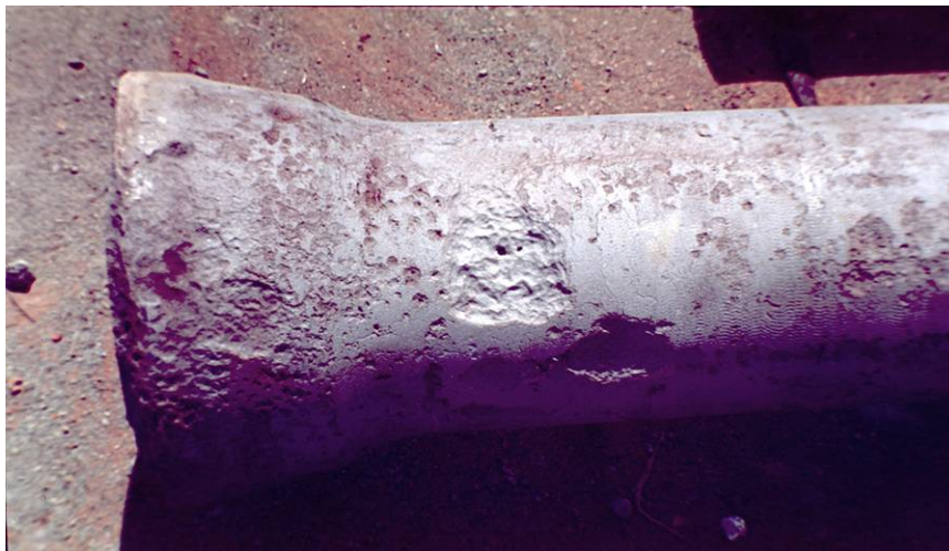
Figure 19 Vancouver, BC, 445 Feet Removed and Examined in Three Sections, Replaced with Tape Coated DIP with Cathodic Protection
