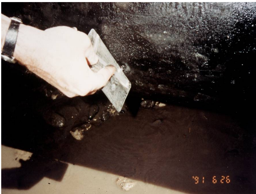
Figure 22 Sheridan, Wyoming, Polyethylene-encased Ductile Iron Pipe With Major Pit at 3 O' Clock, 180 Mils in 340 Mil-Thick-Pipe Wall 14-Year Burial
