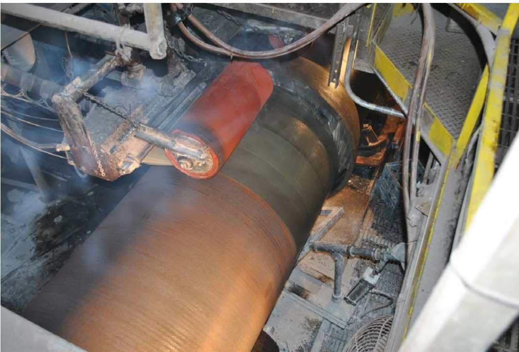
Figure 50 Extruded Polyethylene (Pritec) Ductile Iron Coating Application
