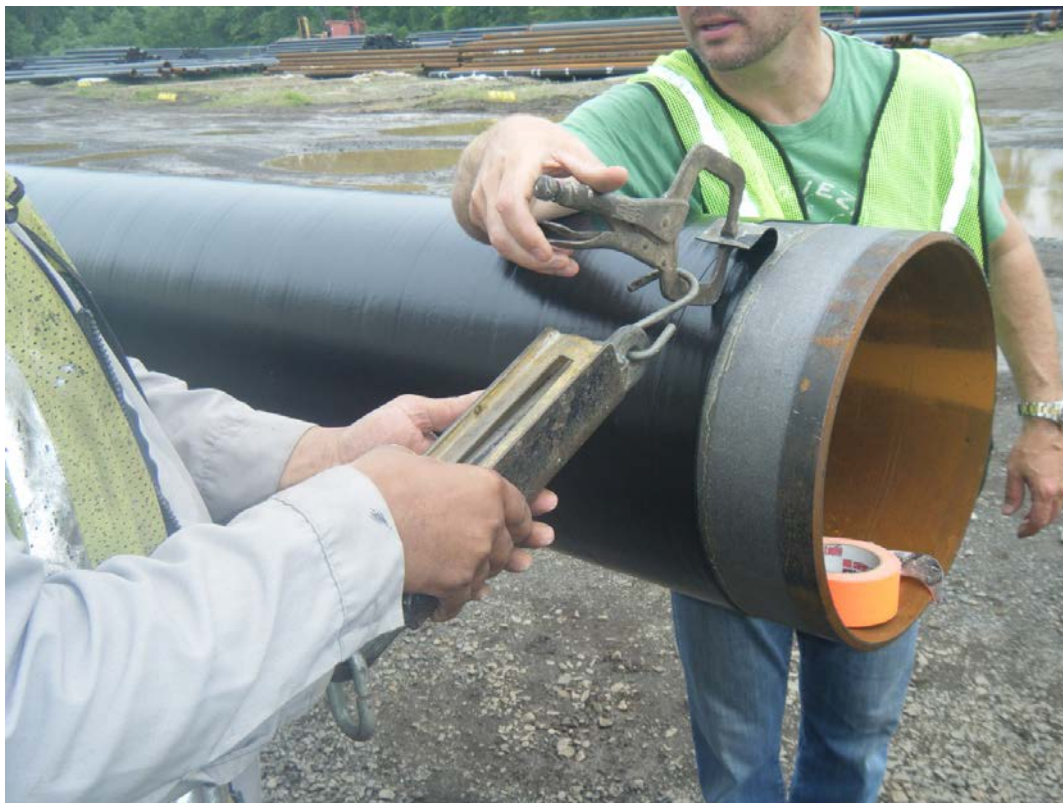
Figure 52 Adhesion Testing of Extruded Polyethylene Coating at Ductile Iron End Cut Back
