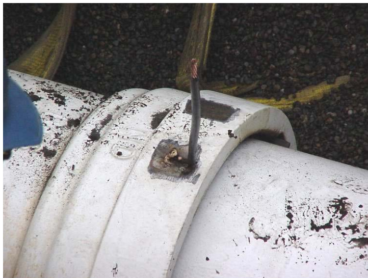
Figure 61 2000 Seattle Thermoplastic Pipe Coating Allows Engagement of Spigot Directly into Bell
