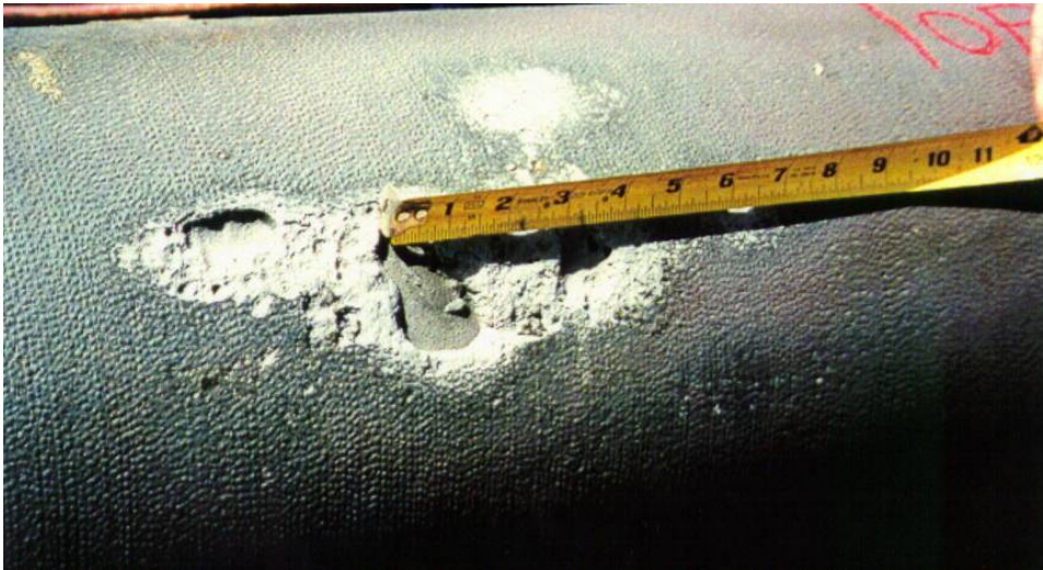
Figure 27 Colorado Springs, Colorado, Force Main Corrosion Where Only Polyethylene Lining Was Holding Sewage Pressure
